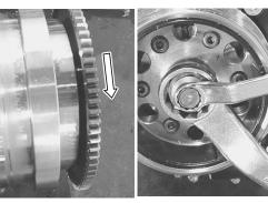
• Install the starter driven gear and the idle gear.
