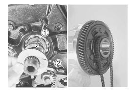
• Install the primary driven gear assembly and engage the chain with the oil pump driven gear.
