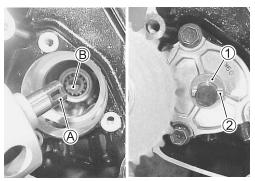
• Install the oil pump driven gear and the circlip.
