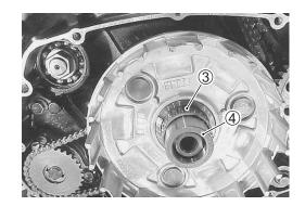
• Install the thrust washer ⑤ and the clutch sleeve hub.
