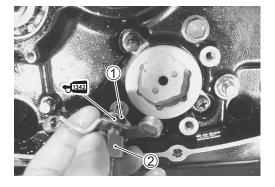
• Install the cam driven gear ① after installing the springs, pins and gearshift pawls.
