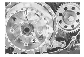
• Tighten the clutch sleeve hub nut to the specified torque with the special tool.
