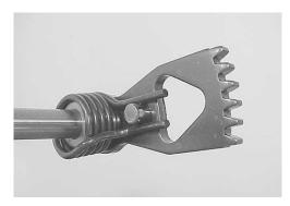
• Install the gearshift shaft with the center of shift gear on the shaft aligned the center of gearshift cam driven gear.
