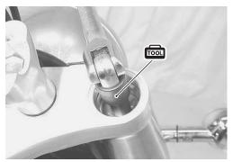
• Remove the front forks after loosening the front fork lower clamp bolts.
