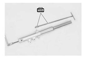
• Remove the damper rod ® and Rebound spring 9.
