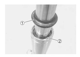
• Remove the oil seal by slowly pulling out the inner tube. NOTE:
