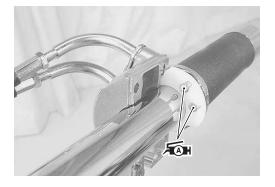
• Install the front brake master cylinder. (\$\sumsymbol{17}7-17\$)
