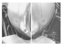
• Remove the cooling air guide.
