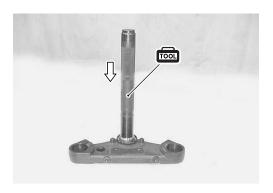
Apply grease to the upper and lower bearings before remounting the steering stem.
