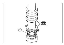
• Install the oil seal stopper ring 2.
