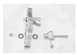
• Remove the handlebar bushes by using the proper tool and special tools.
