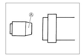
• Insert the inner tube into the outer tube and install the oil seal ① using the special tool.
