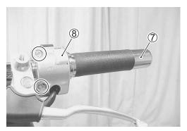
• Remove the handlebars by removing the handlebar clamp bolt caps, handlebar clamp bolts and handlebar clamps.
