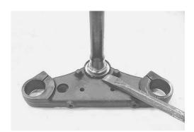
• Drive out the steering stem upper and lower bearing races by using the special tools and suitable bar.
