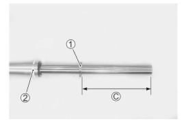
• Install the inner tube cover ①, rubber ② and washer ③.
