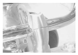
• First, tighten the handlebar clamp bolts ① to the half of specified torque, and then tighten the handlebar clamp bolts ① and ② to the specified torque.
