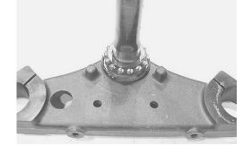
• Remove the steering stem lower bearing inner race by using a chisel.
