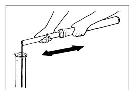
• Remove the damper rod bolt using a 6-mm hexagon wrench and the special tools.
