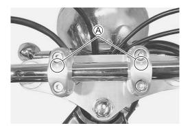
• Install the handlebars with the punch mark ® aligned with the handlebar clamp as shown.
