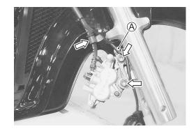
• Remove the front fender by removing its mounting bolts.
