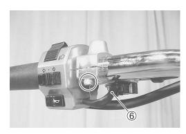
• Remove the left handlebar balancer  $\overline{\mathcal{T}}$  and the left handlebar switch  $\underline{\$}$ .
