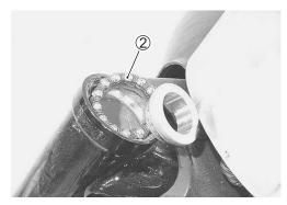
• Remove the steering stem lower bearing ③.
