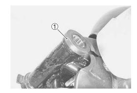
• Remove the steering stem upper bearing 2.
