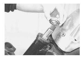
Tighten the steering stem nut to the specified torque using the special tools.
