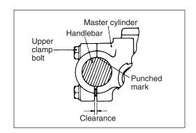
• Install the clutch lever holder with the punch mark (A) aligned with the clutch lever holder clamp as shown.
