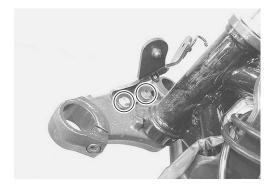
• Remove the steering stem nut using the special tool.
